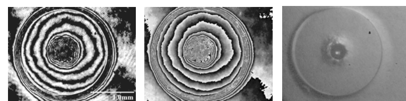
Unloading: Fringe pattern, wrapped phase and contact radius
