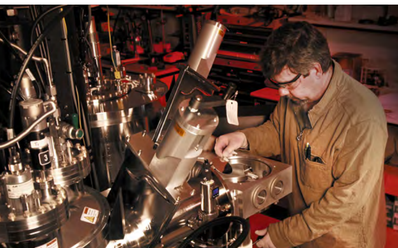
CINT Technologist Kevin Baldwin makes samples on the Physical Vapor Deposition System.
