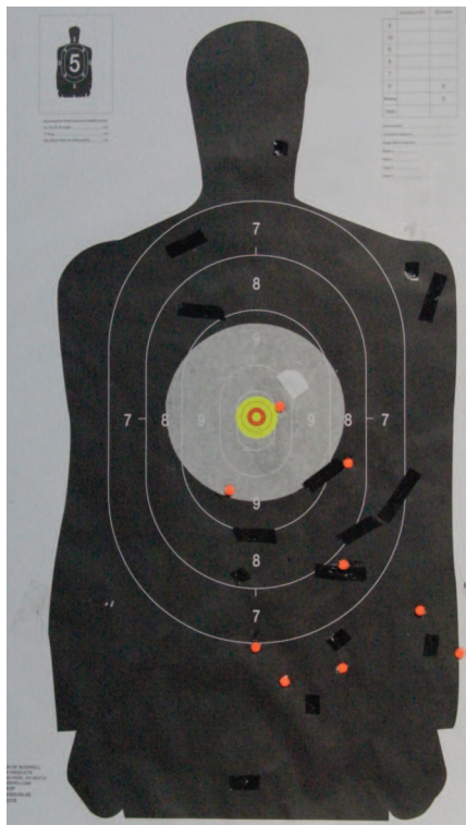
Battelle non-lethal ballistic system demonstration. A 10 shot group was fired outdoors from the prone position at 115 yards (one of the 10 shots hit below the target).
