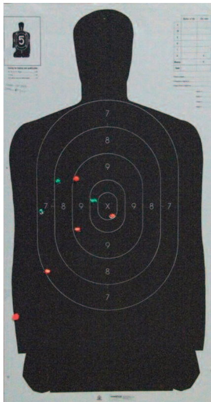
Battelle non-lethal ballistic system demonstration at an indoor range. Green ear plugs are off hand shots at 35 and 65 yards, and the orange ear plugs are off-hand, sitting shots taken from 100 yards.
