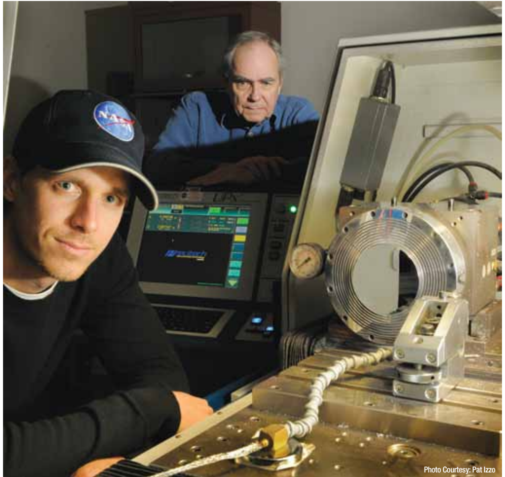
Technologists Peter Hill (foreground) and Vince Bly pose with a single-crystal silicon mirror, which is mounted in the mandrel of the diamond-turning machine used in its fabrication.
