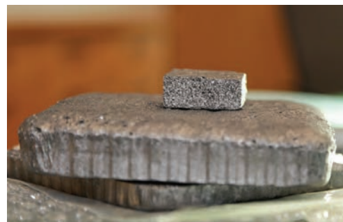
Graphite foam, invented by ORNL's James Klett, was key in cooling the Large Hadron Collider's ATLAS detector. (Photo: Jason Richards)
