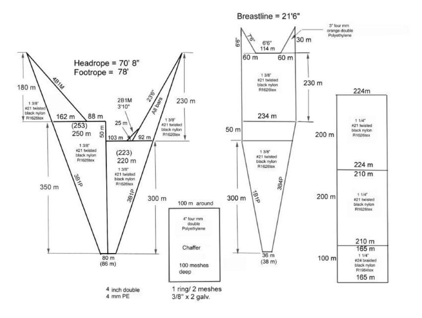
Numbers in parentheses (##) are the actual number of meshes in the section. The additional meshes are wrapped in the gore, Meshe sizes are knot center to knot center.
