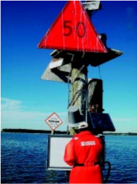
Figure 7. USGS servicing of estuary monitoring platform. These monitoring systems provide real-time data on dissolved oxygen, salinity, and temperature; the data are used by researchers, State resource managers, fishermen, and the public.
