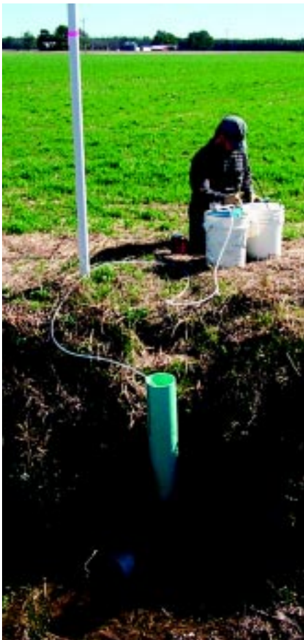
Figure 5. Water sample being collected from a tile drain beneath cropland. Water from the tile drain typically flows into the drainage ditch and subsequently to a stream. High nutrient loadings from cropland can have undesirable effects on surface-water quality.
