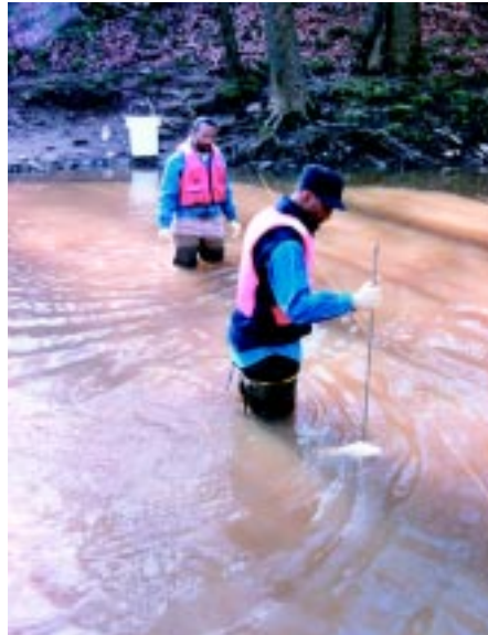
Figure 3. Stream-water sample being collected by the USGS. Water is collected throughout the channel cross section to ensure that a representative sample is obtained. Ultra-clean methods are used to avoid environmental contamination of the water sample.
