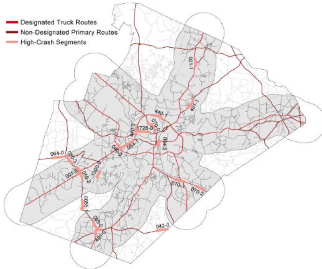
Figure 3. High truck crash segments that were identified using the Corridor Analysis program, including three segments outside of the designated truck zone.
