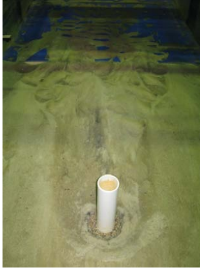
Figure 57. Photo. Result of a pier scour test with a graded sediment.
