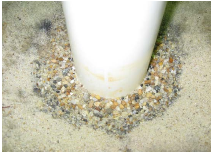
Figure 58. Photo. Result of a pier scour test showing the armoring layer.
