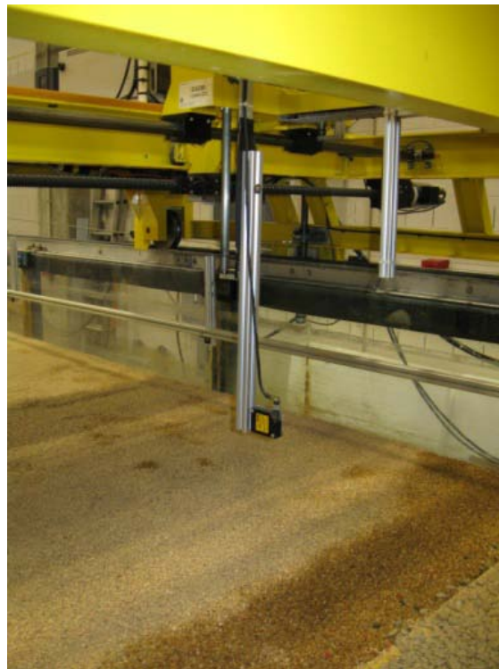
Figure 54. Photo. Automated point laser distance sensor (side view).
