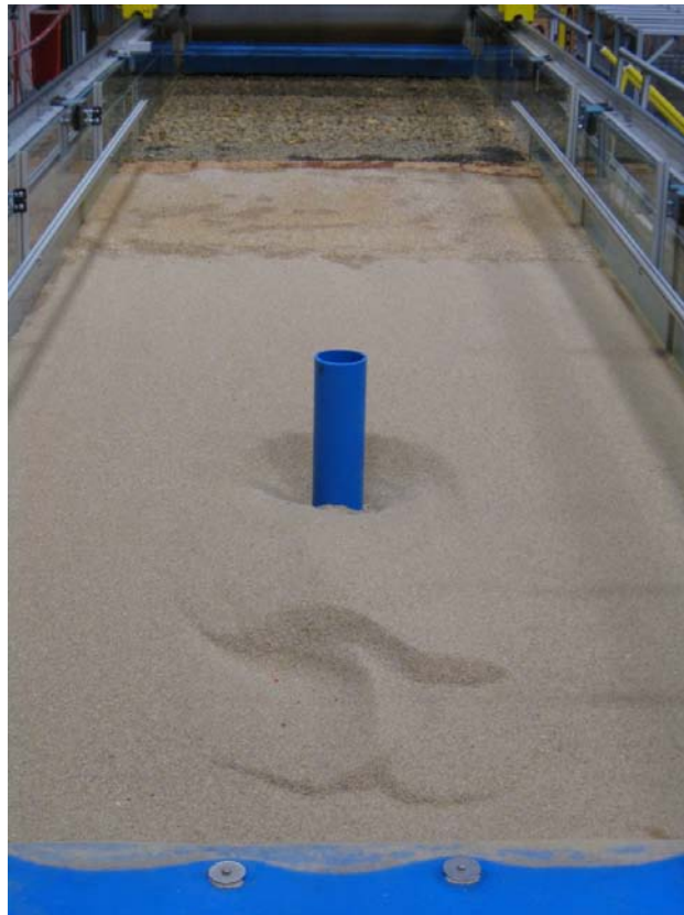
Figure 56. Photo. Bed bathymetry after a pier scour test.
