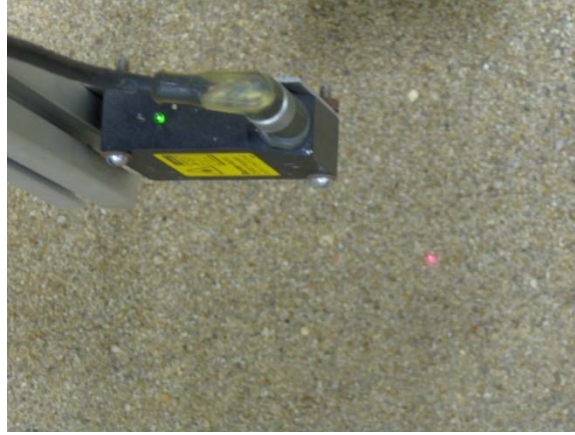
Figure 55. Photo. Automated point laser distance sensor (top view).
