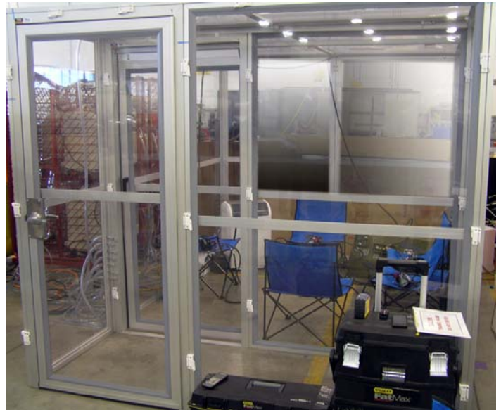
PROTE chamber can accommodate five trainees for a ground-base excursion to 25,000 feet.
