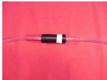
Figure 4-4c. Asbestos Cassette in-line
