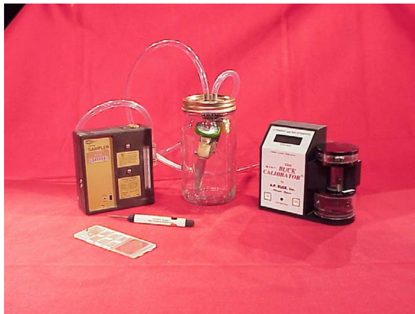
Figure 4-5. Mini-Buck Wet Bubble Calibrator Set-up for Calibration
