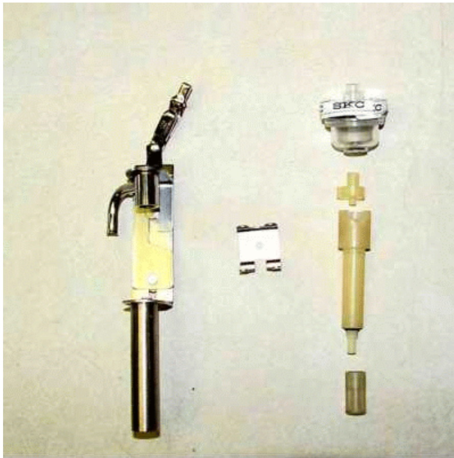
Figure 22-1. DPM Cassette, Cyclone and Holder Assembly
