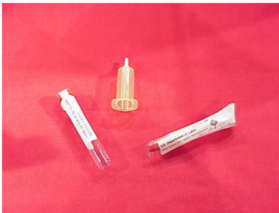
Figure 12-2. 10 mL Vacutainer, Plunger, and Sealed Sample
