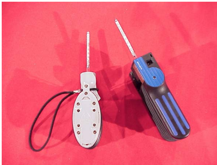
Figure 11-3. Detector Tube and Bellows-Type Pump Systems
