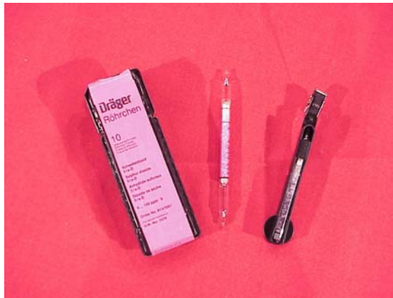
Figure 11-2. Diffusion Tube and Holder
