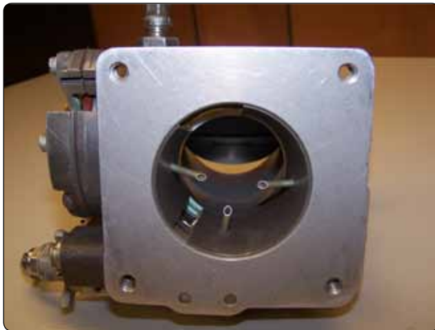
Figure 2-32. Impact tubes for inlet air pressure.
