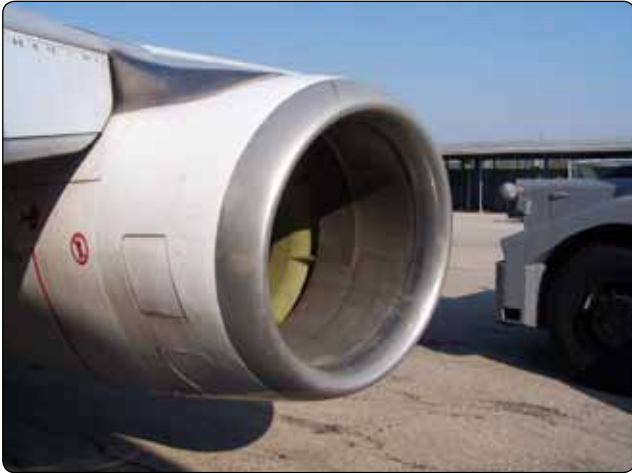
Figure 3-34. A typical turbofan intake section.
