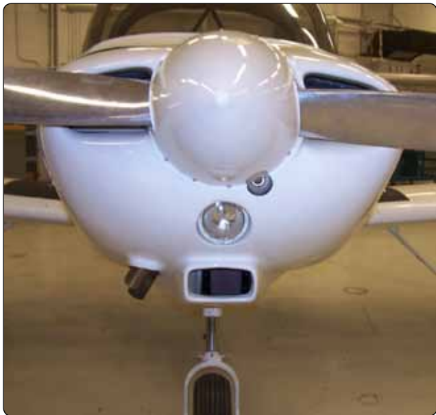
Figure 3-1. Inlet scoop in engine cowling.
