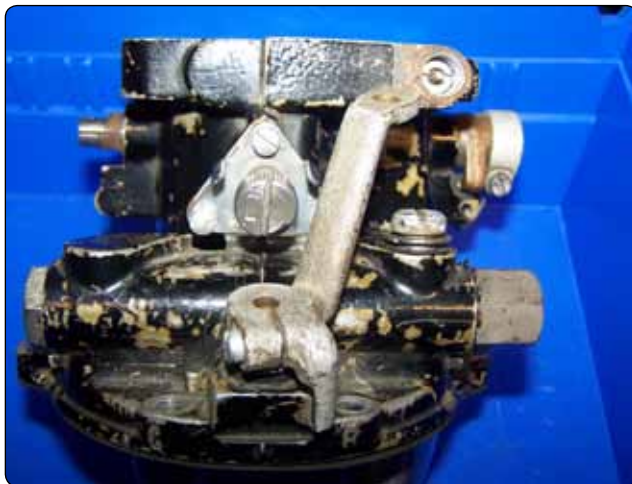
Figure 2-46. Idle mixture adjustment for carburetor.
