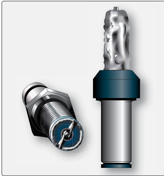
Figure 4-49. Lead fouled spark plug.
