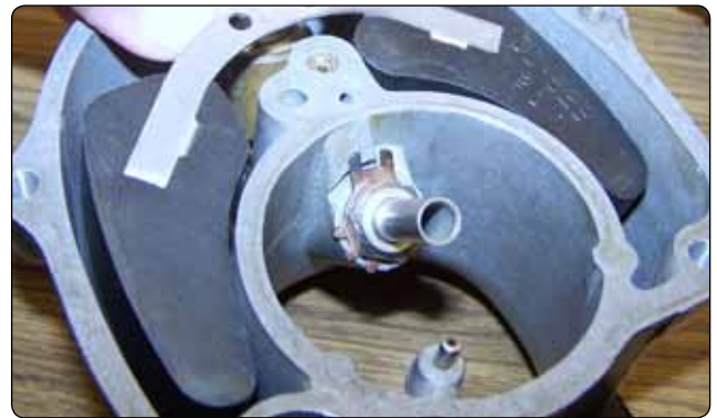
Figure 2-9. Float chamber discharge nozzle and float.
