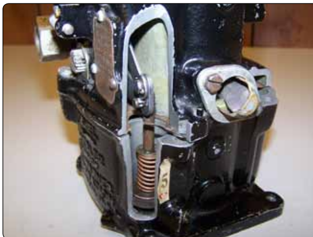
Figure 2-19. Accelerating pump shown in cutaway.
