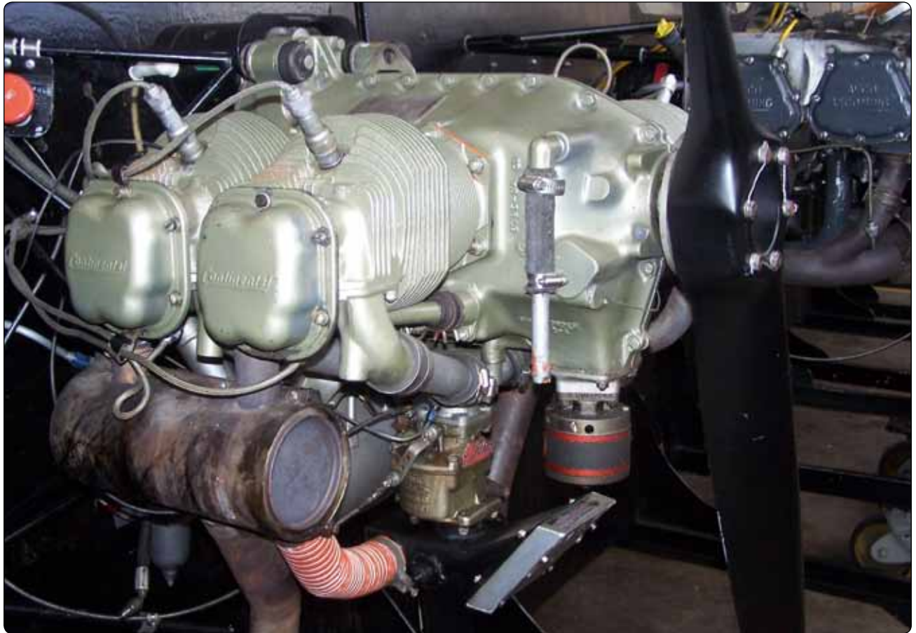
Figure 3-9. An example of a naturally aspirated reciprocating engine.
