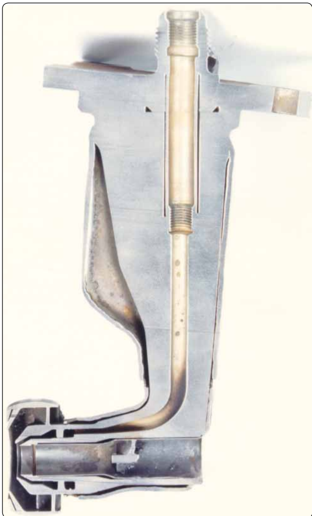
Figure 2-64. Simplex airblast nozzle cutaway.
