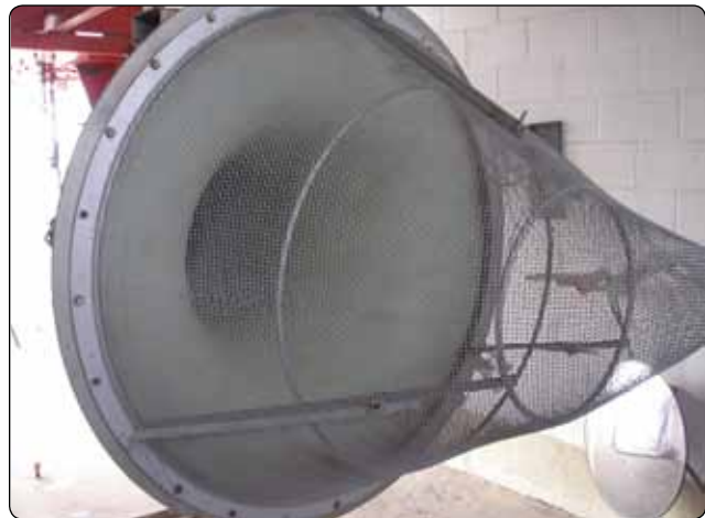
Figure 3-30. A bellmouth inlet used during system tests.
