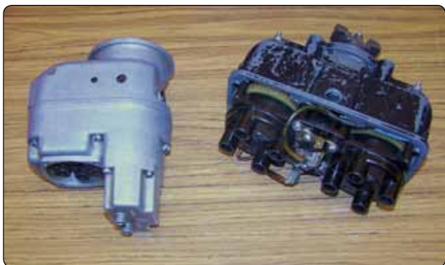
Figure 4-1. Single and dual magnetos.
