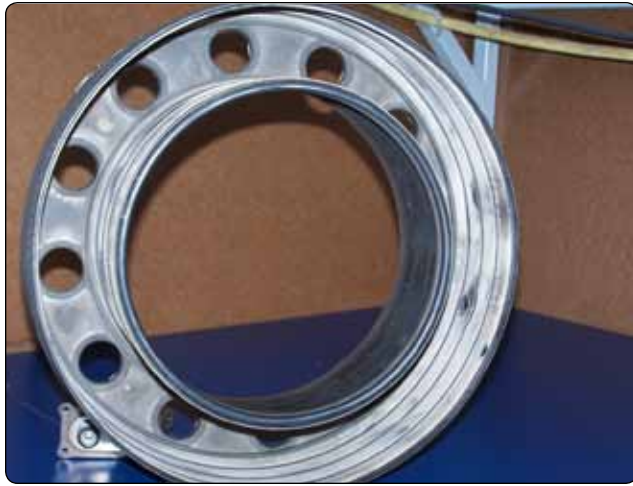
Figure 1-58. Annular combustion with chamber ceramic coating.
