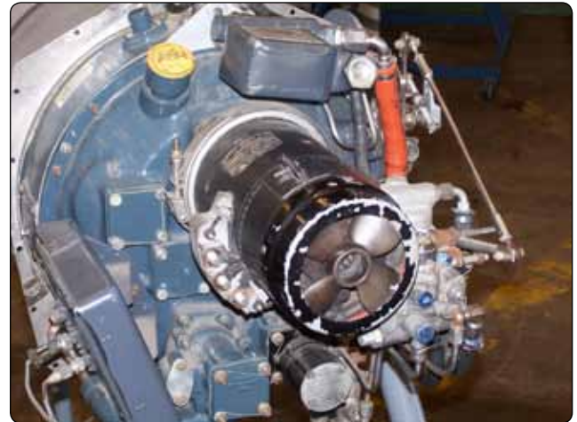
Figure 1-45. Typical turboprop accessory case.
