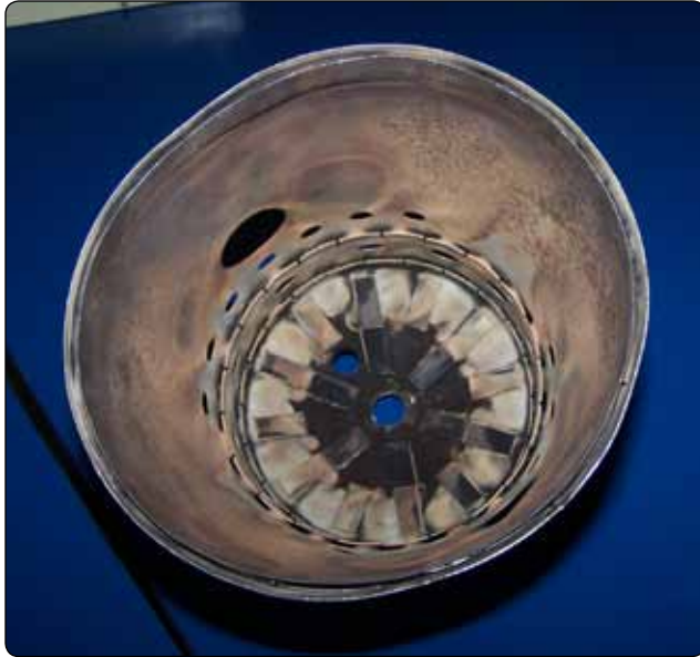
Figure 1-53. Inside view of a combustion chamber liner.
