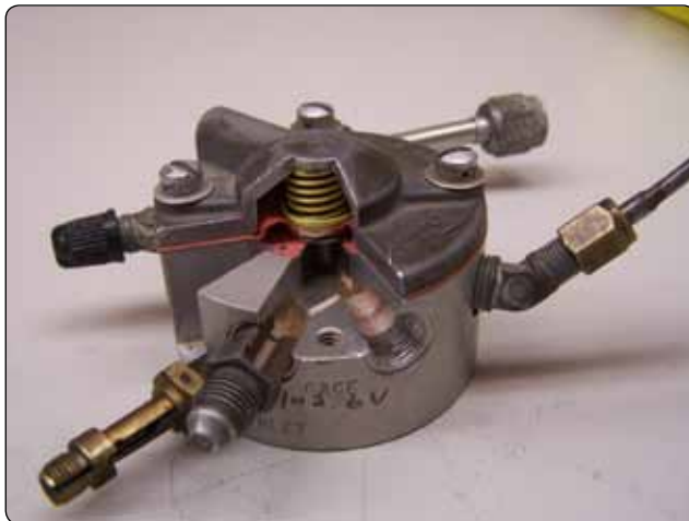
Figure 2-37. Flow divider cutaway.
