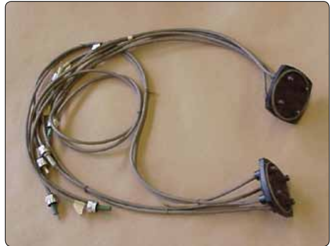
Figure 4-22. Typical six-cylinder engine electronic control and low-voltage harness.
