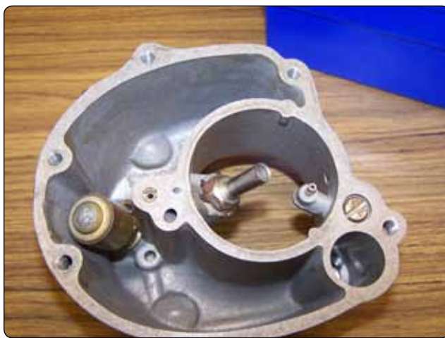
Figure 2-11. Float chamber (bowl) with float removed.
