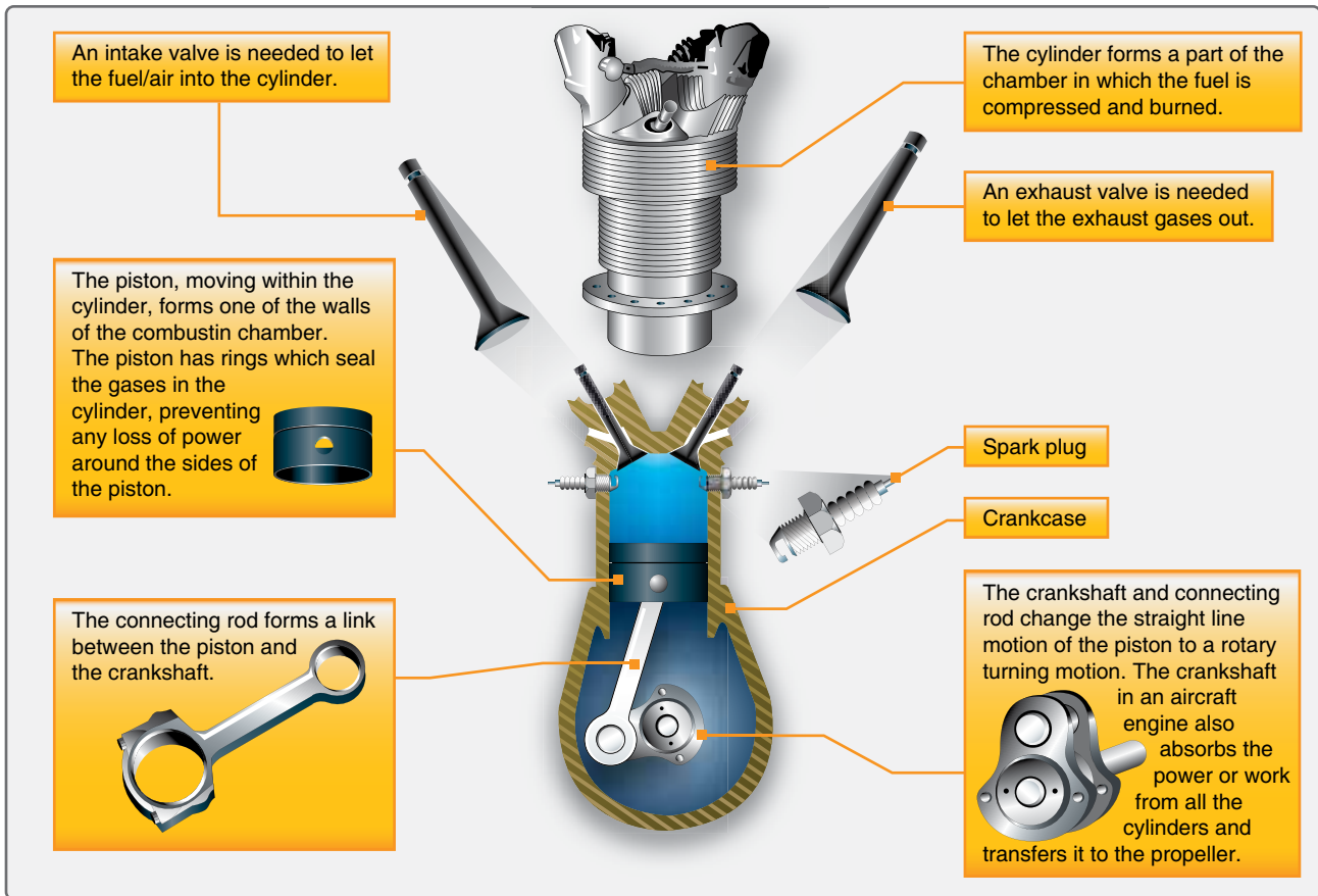
Figure 1-4. Basic parts of a reciprocating engine.
