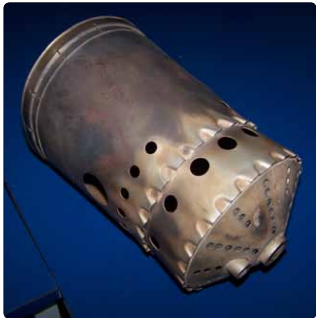
Figure 1-52. Can-type combustion chamber.
