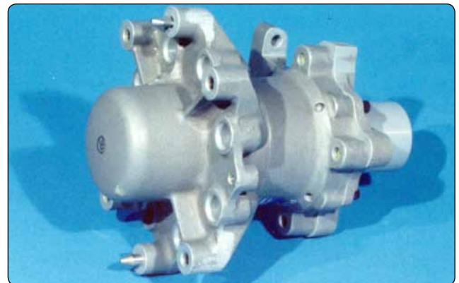
Figure 2-58. Fuel distribution valve.
