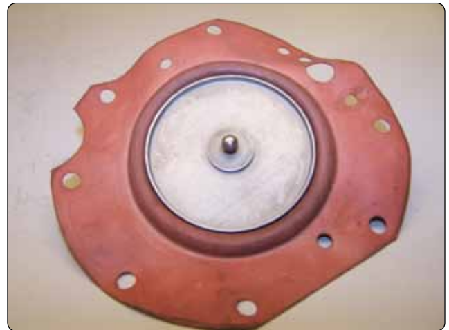
Figure 2-33. Fuel diaphragm with ball valve attached.
