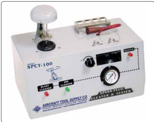
Figure 4-55. Spark plug cleaner tester.
