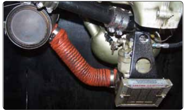
Figure 3-5. Location of a carburetor heat air valve.
