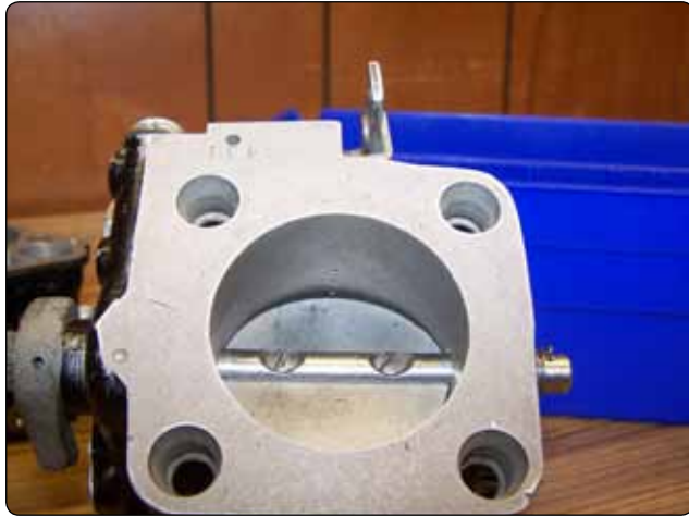
Figure 2-14. Throttle action in idle position.
