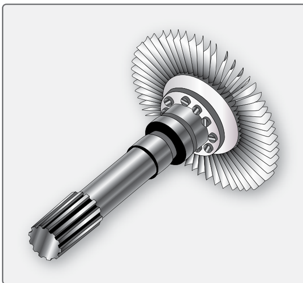
Figure 1-63. Rotor elements of the turbine assembly.
