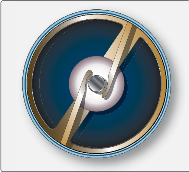
Figure 4-50. Spark plug gap erosion.
