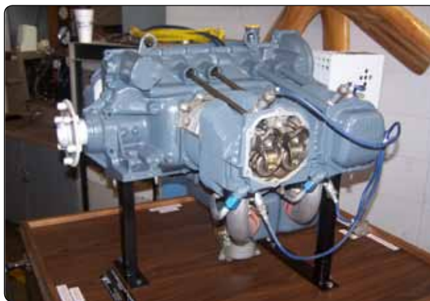
Figure 1-1. A typical four-cylinder opposed engine.
