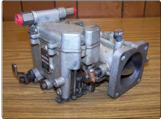
Figure 2-5. Side draft horizontal flow carburetor.
