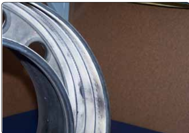
Figure 1-55. Annular combustion chamber liner.
