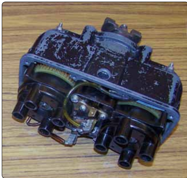
Figure 4-18. A dual magneto with two distributors.
