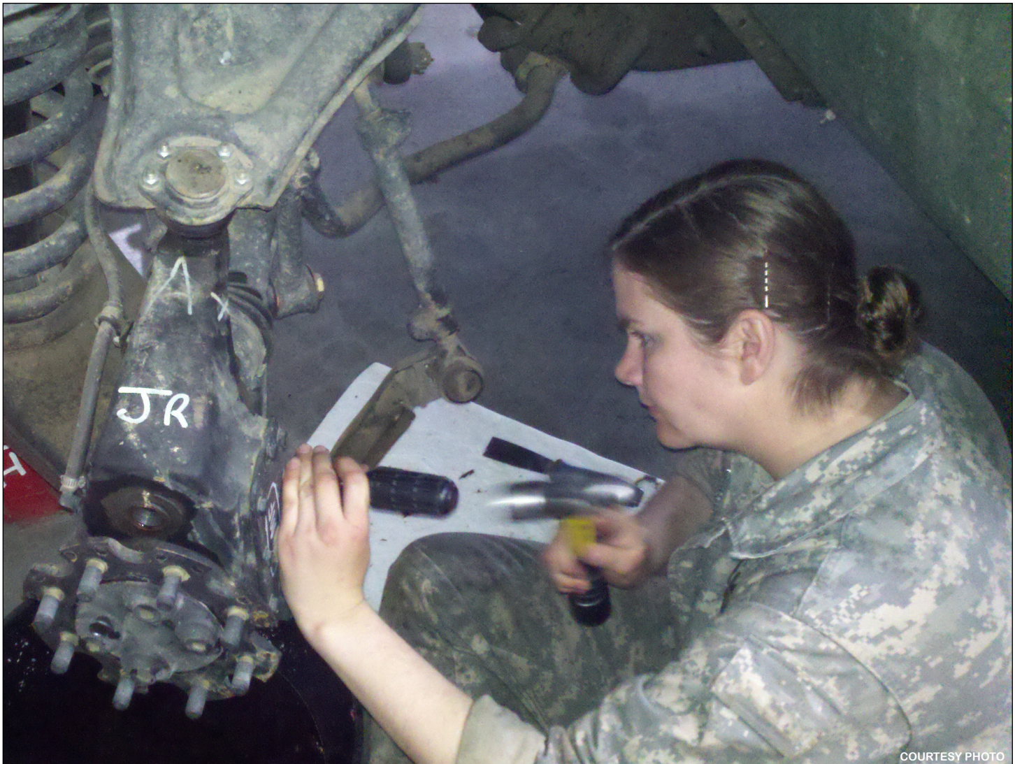
Cpl. Samantha Sherman, a wheeled vehicle mechanic assigned to the 542nd Support Maintenance Company, 80th Ordnance Battalion, 593rd Sustainment Brigade, and a native of Brule, Neb., changes a hub seal while performing an annual service on an M1097 at Fort Wainwright, Alaska, on 3 June 2011.
