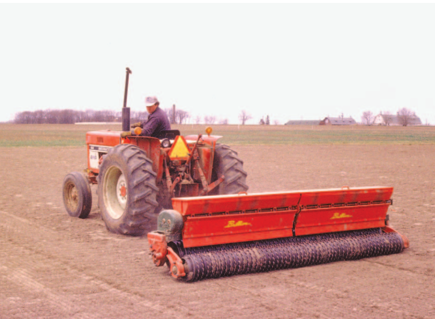
A cultipacker-type seed drill used for a spring seeding in Ohio. Seed is dropped between the front and back rollers, which are offset slightly so the back roller covers the seed. Credit: Mark Sulc, The Ohio State University.
