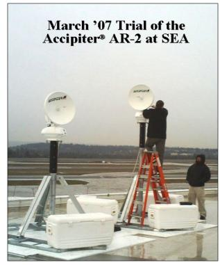
Building for two weeks in March 2007. The purpose of this trial was to verify that this location offered minimal interfering radar "clutter" and to test for potential interference with the FAA's ASDE-X ground radar system. With the success of this first phase, the final design was completed and approved in time for a June construction date.
