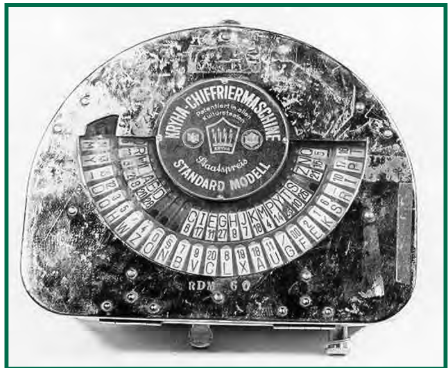
The clockwork-driven Kryha, a popular German-made cipher machine that was widely used commercially in the 1930s
