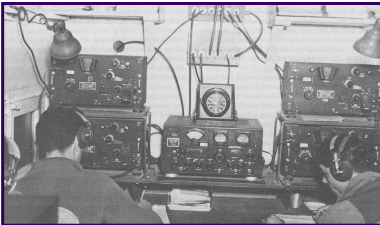
849th SIS Mediterranean Theater (3916th Signal Service Company) intercept van with double bank of receivers (BG 342 and BC 344) and the S-36 (VHF) in the middle (Photograph from the NSA History Collection)
