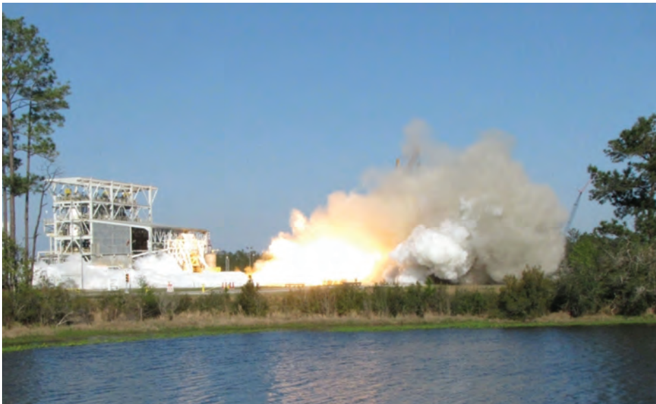
A team of engineers from NASA's John C. Stennis Space Center, Orbital Sciences Corporation, and Aerojet conducts a successful test of an Aerojet AJ26 rocket engine on 19 March. Stennis is testing AJ26 engines for Orbital Sciences to power commercial cargo missions to the International Space Station.
