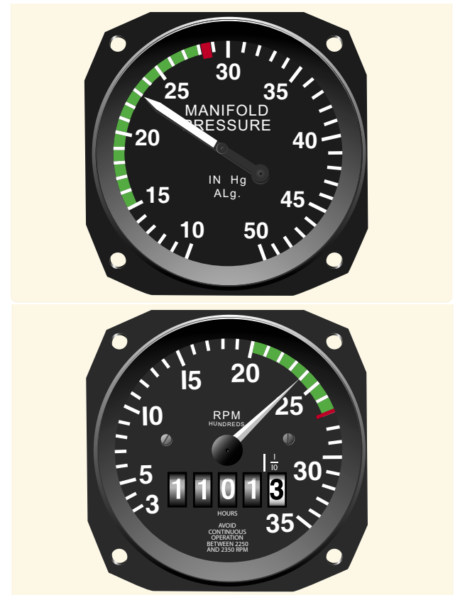
Figure 8-4. Manifold pressure gauge (top) and tachometer (bottom).
