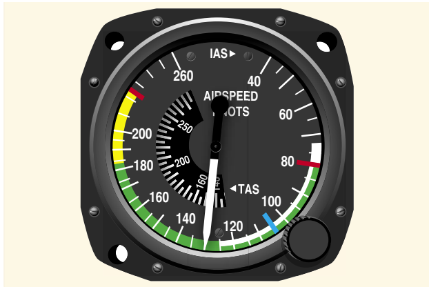
Figure 8-2. Multi-engine airspeed indicator.
