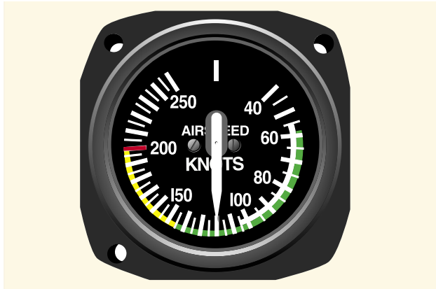
Figure 8-1. Single-engine airspeed indicator.
