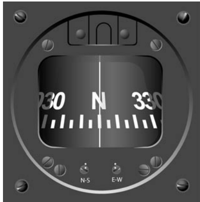
Figure 7-31. A magnetic compass. The vertical line is called the lubber line.
