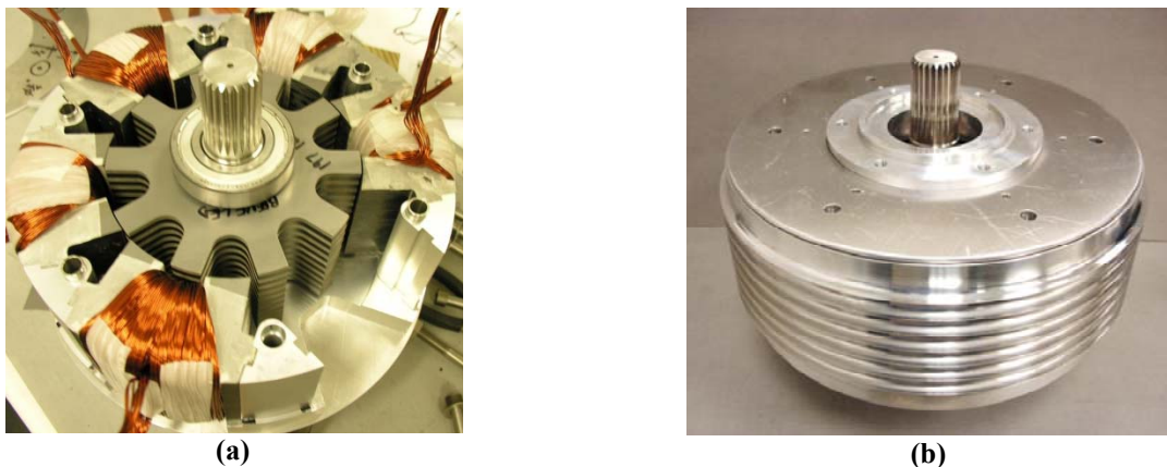
Fig. 8. IMFP SRM final assembly: (a) winding installation and (b) finished IMFP SRM.
