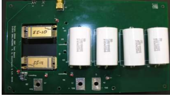
Power Board used for Testing
