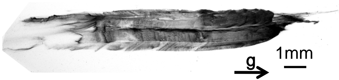
Figure 7. SWBXT image of 8-hour Fiber 2 crystal. The central faceted sections where no 3C-SiC has nucleated are epitaxial with the substrate and are of high crystalline quality and low strain.
