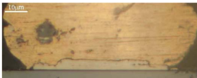
Figure 6. Intermetallic formation between Au wire and Al bond pad
