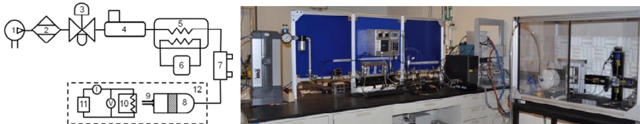
Figure 8. Schematic and photograph of the steady jet experimental setup: (1) compressed air, (2) desiccant dryer, (3) filter/regulator, (4) mass flow controller, (5) plate heat exchanger, (6) recirculating bath, (7) laminar flow element, (8) settling chamber, (9) nozzle, (10) heater target, (11) heater power supply, (12) isolation box
