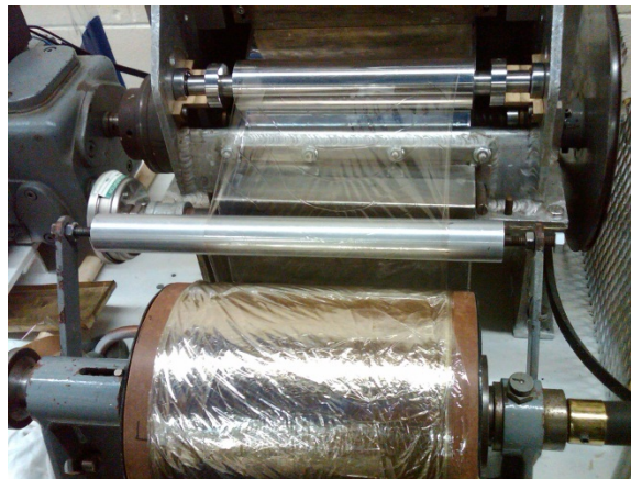
Figure 9. Casting of hydrogenated polymer with stoichiometry n = 3m at ECI
