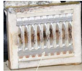
•Lack of compression in louvered contact led to arcing between circuit card and busbar contact
