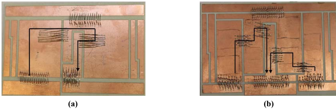
Fig. 15. Fabricated commutation loops for (a) the conventional design and (b) the proposed design.
