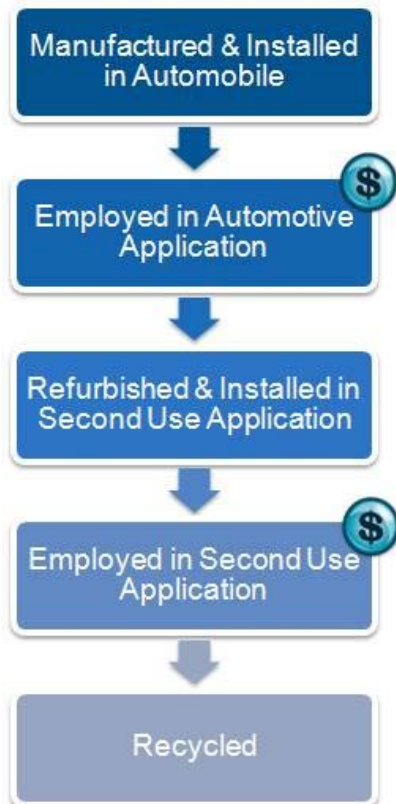
Figure 1: Lifetime of a PHEV/EV battery when second-use applications are considered to increase its total lifetime value
