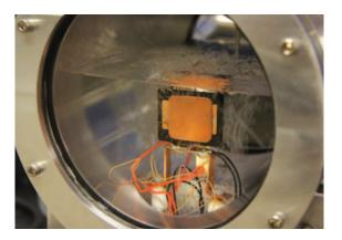
NREL is developing improved cooling systems for the power electronics devices in hybrid and electric vehicles. Researchers are enhancing the surfaces of these devices with microporous coatings to accelerate the transfer of heat to the surrounding coolant. This two-phase system has demonstrated a fivefold improvement in heat transfer relative to traditional systems, potentially yielding a system with a lower weight, volume, and cost.
