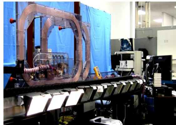
Fig. 4. ORNL laboratory test apparatus with alignment-adjustable antennas for wireless power transfer.
