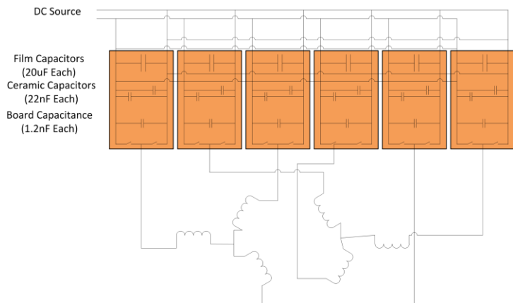
Fig. 8. Controller architecture for demonstrator 10 kW IMMD drive.
