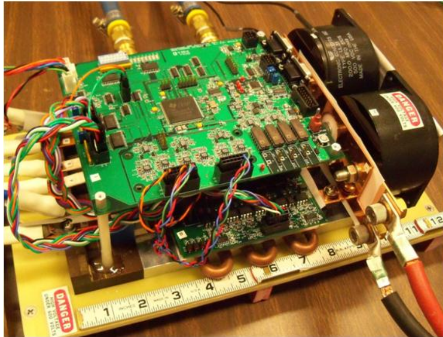
Fig. 6. A 55 kW segmented inverter prototype.
