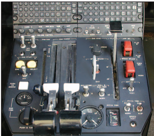
Figure 15-3. Jet engine power controls.
