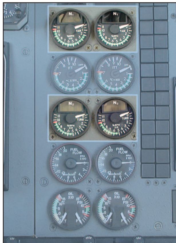
Figure 15-4. Jet engine r.p.m. gauges.
