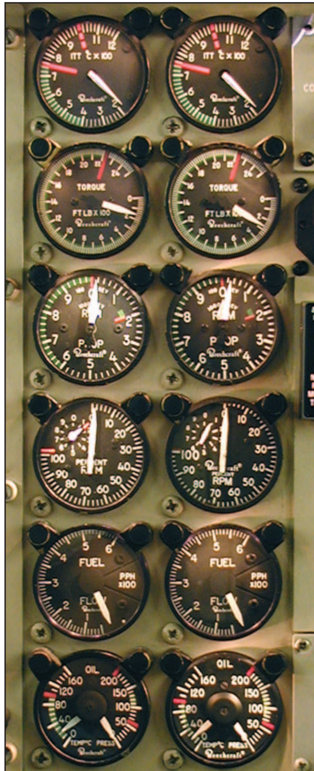
Figure 14-7. Engine instruments—split shaft/free turbine engine.
