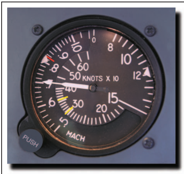
Figure 15-8. Jet airspeed indicator.
