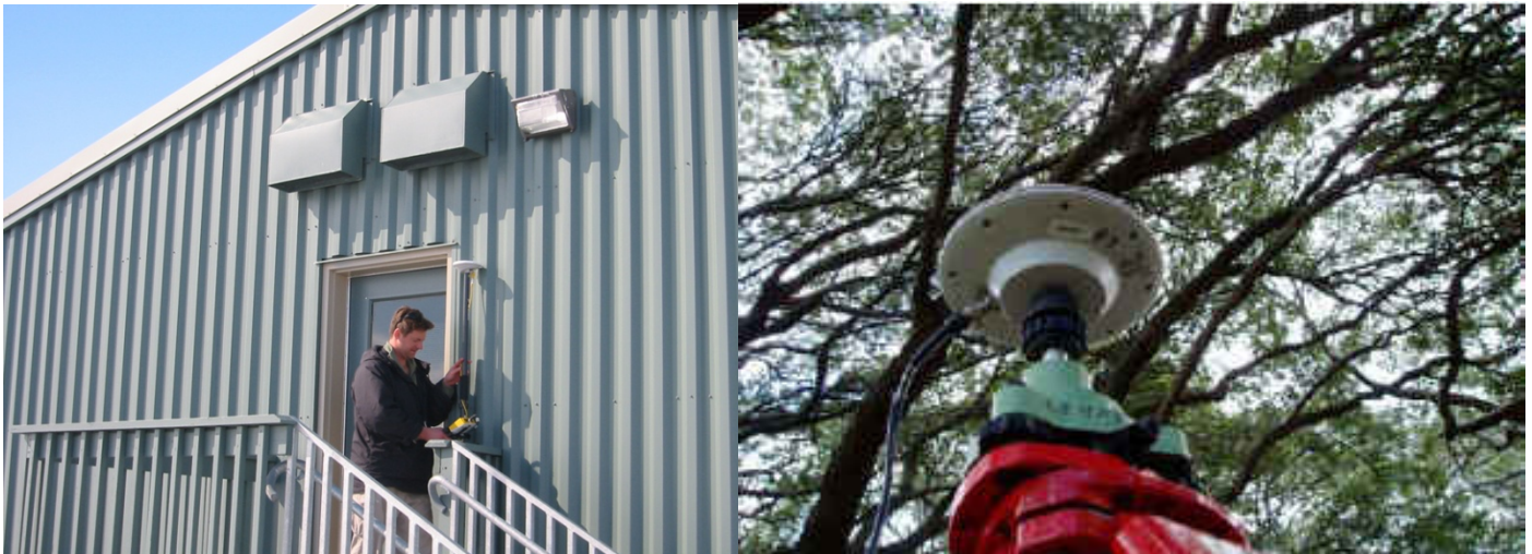
Multipath Conditions can cause unacceptable errors by introducing noise and incorrect ambiguity resolution because of signal delay.
