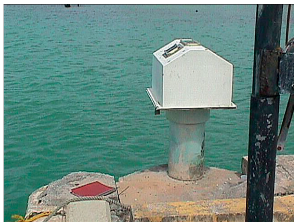
Figure 11. Tide gage (NWLON site #1633227) at Tanapag Harbor, Saipan, CNMI.
