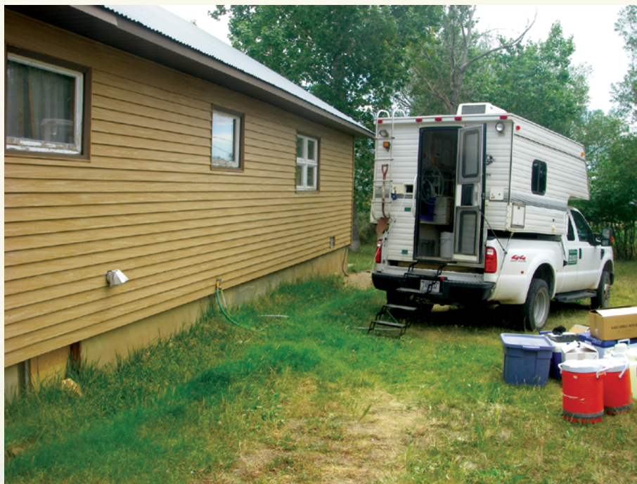
Figure 2. Mobile water-quality laboratory used for the collection of samples from groundwater wells.
