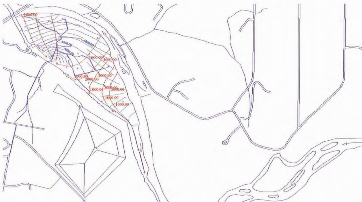
Figure 4-46. Results of Particle Tracking Simulation for Floodplain Alluvial Aquifer, Shiprock, New Mexico UMTRA Site. Arrowheads Indicate 1,000-Days Travel Time For Fluid Elements.
