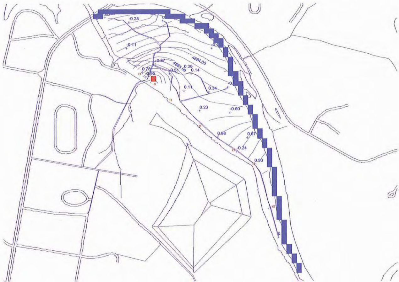
Figure 4-45. Hydraulic Head and Residuals from Calibrated Flow Model of Floodplain Alluvial Aquifer at the Shiprock, New Mexico UMTRA Site
