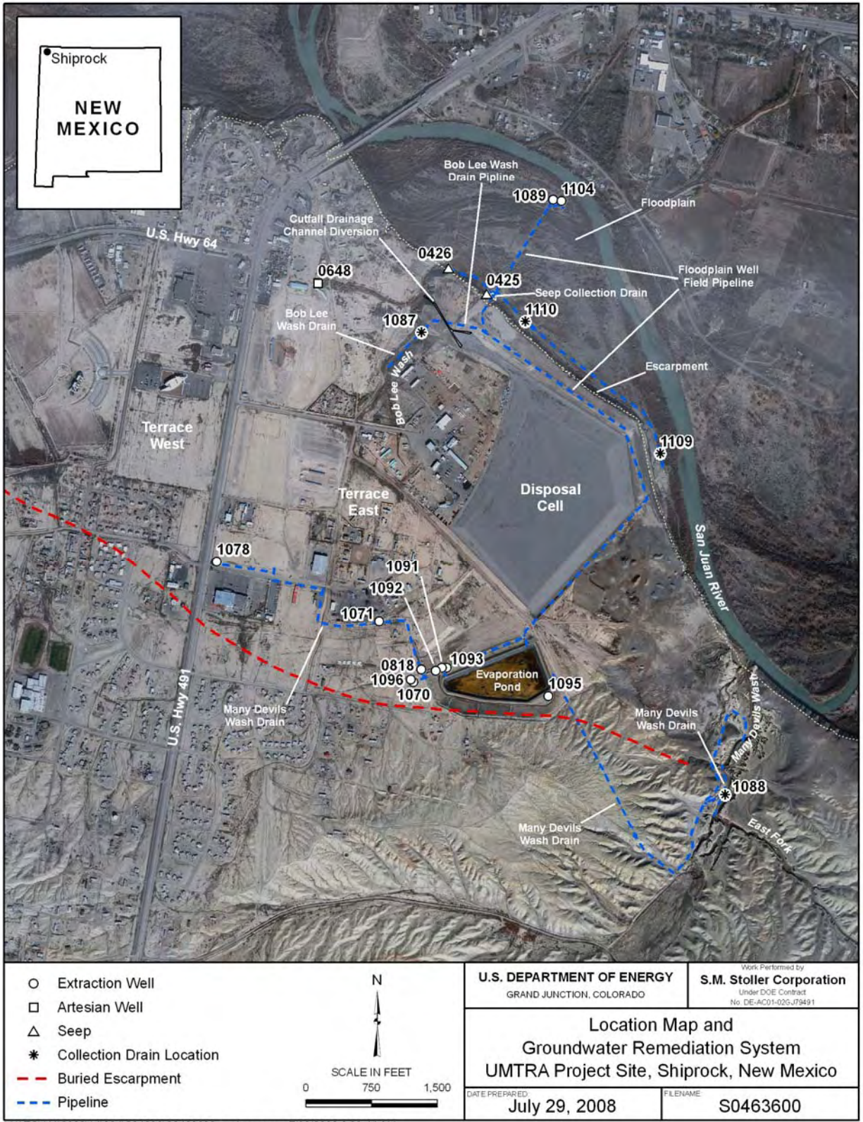
Figure 1-1. Location Map and Groundwater Remediation System
