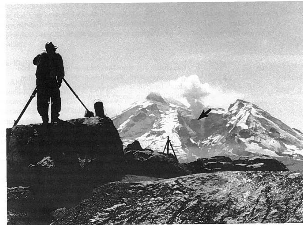
Measuring the growth rate of a lava dome (arrow) at Redoubt Volcano, Alaska. Scientists use various methods to track the rate of magma supply to a growing dome. In this photograph, a scientist peers through a theodolite, an instrument that precisely measures horizontal and vertical angles, to estimate changes in the dome's rate of growth. Photograph by R.G. McGimsey.
