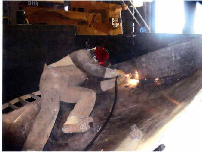
Figure 2. Welder Removing Bulldozer Blade Wear Plates
