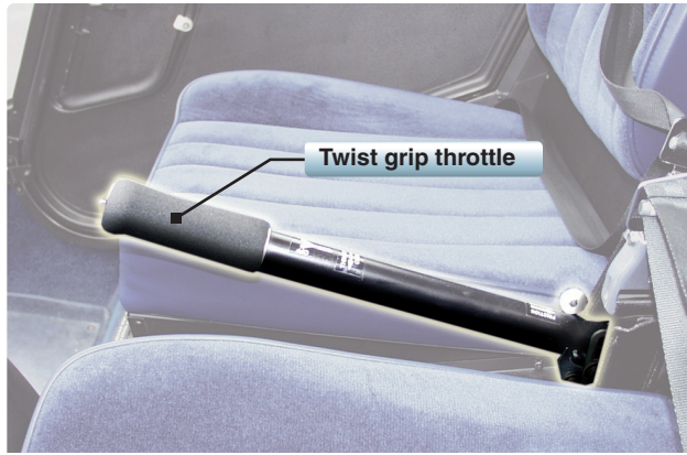
Figure 3-2. A twist grip throttle is usually mounted on the end of the collective lever. The throttles on some turbine helicopters are mounted on the overhead panel or on the floor in the cockpit.
