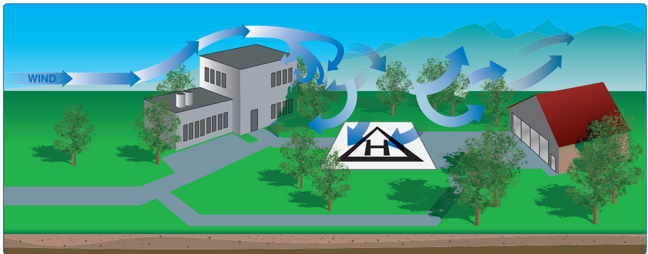
Figure 10-8. If the wind velocity is 10 knots or greater, expect updrafts on the windward side and downdrafts on the lee side of obstacles. Plan the approach with these factors in mind, but be ready to alter plans if the wind speed or direction changes.
