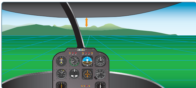
Figure 9-10. Maintain straight-and-level flight by adjusting the rotor tip-path plane forward but adjusting the collective as necessary to maintain a constant airspeed and altitude. The natural horizon line can be used as an aid in maintaining straight-and-level flight. If the horizon line begins to rise, slight power may be required or the nose of the helicopter may be too low. If the horizon line is slowly dropping, some power may need to be taken out or the nose of the helicopter may be too high, requiring a cyclic adjustment.
