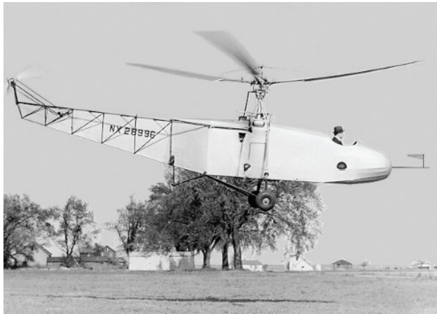
Figure 1-8. Igor Sikorsky designed the VS-300 helicopter incorporating the tail rotor into the design.
