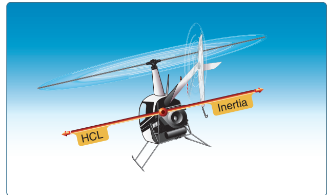
Figure 9-11. During a level, coordinated turn, the rate of turn is commensurate with the angle of bank used, and inertia and horizontal component of lift (HCL) are equal.
