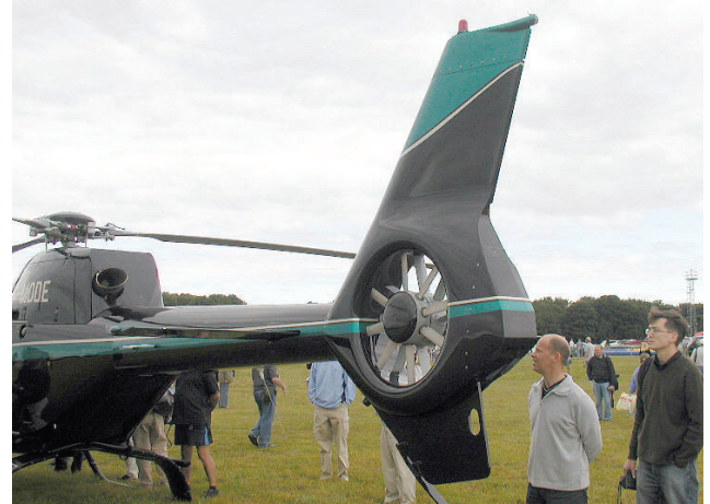
Figure 4-13. Fenestron or “fan-in-tail” antitorque system. This design provides an improved margin of safety during ground operations.
