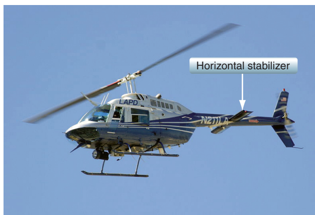
Figure 1-12. The horizontal stabilizer levels the helicopter airframe to minimize drag during flight.
