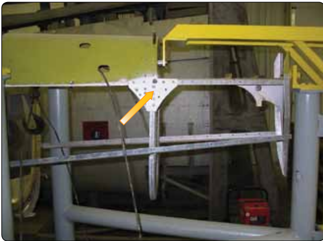
Figure 1-18. Gussets are used to increase strength.
