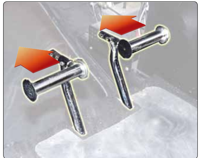
Figure 2-49. Antitorque pedals compensate for changes in torque and control heading in a hover.
