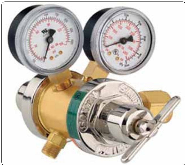
Figure 5-14. Two-stage oxygen regulator. No groove on the cylinder connection nut indicates a right hand thread.
