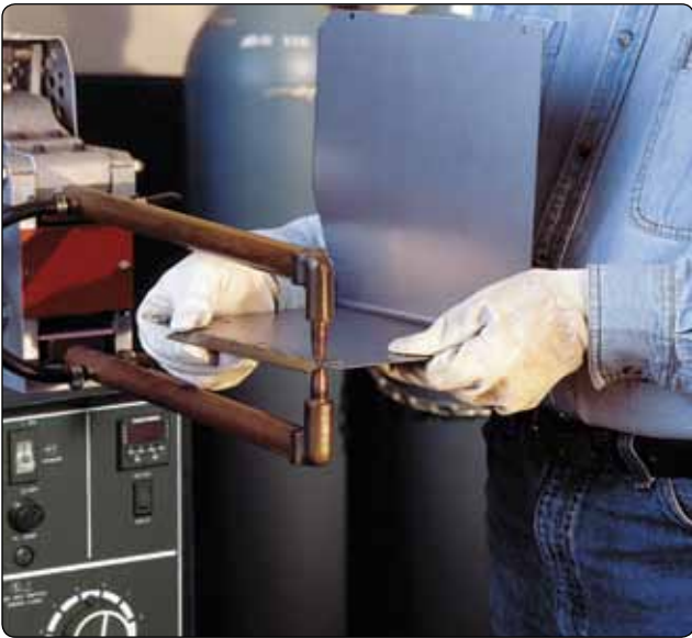
Figure 5-10. Spot welding thin sheet metal.
