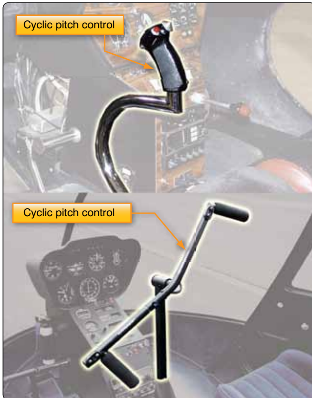
Figure 2-48. The cyclic pitch control may be mounted vertically between the pilot's knees or on a teetering bar from a single cyclic located in the center of the helicopter. The cyclic can pivot in all directions.
