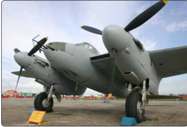
Figure 1-9. The DeHavilland Mosquito, the first aircraft with foam core honeycomb in the fuselage.
