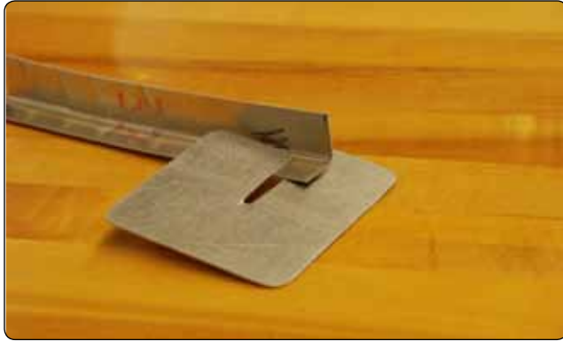
Figure 4-165. Samples of joggled metal.
