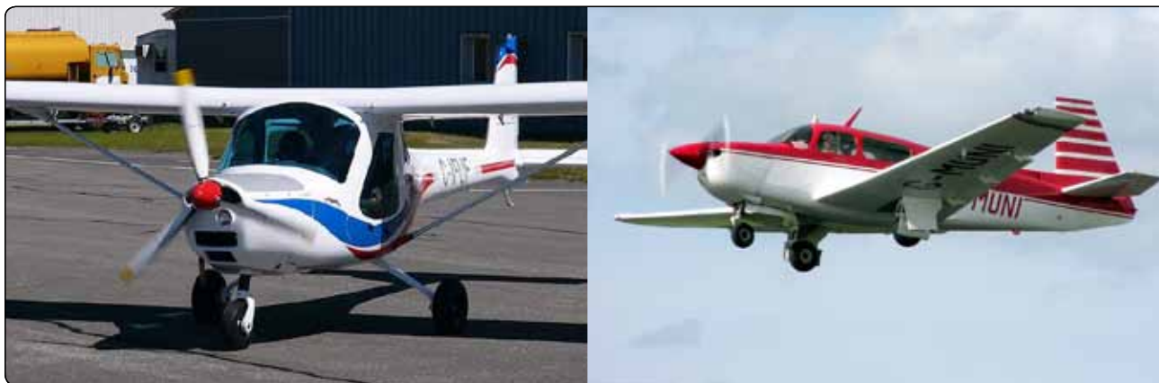
Figure 1-87. Tricycle landing gear is the most predominant landing gear configuration in aviation.
