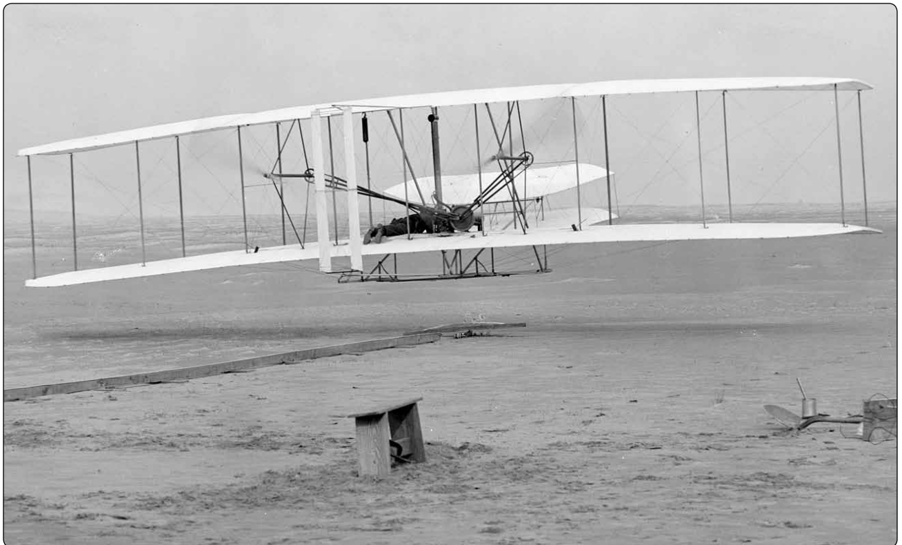
Figure 1-4. The Wright Flyer was the first successful powered aircraft. It was made primarily of wood and fabric.
