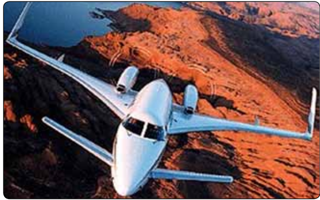
Figure 2-19. The Beechcraft 2000 Starship has canard wings.
