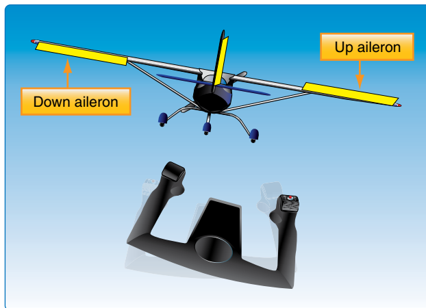
Figure 1-54. Differential aileron control movement. When one aileron is moved down, the aileron on the opposite wing is deflected upward.
