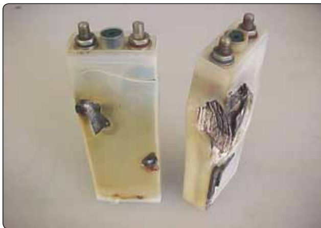
Figure 9-35. Thermal runaway damage.
