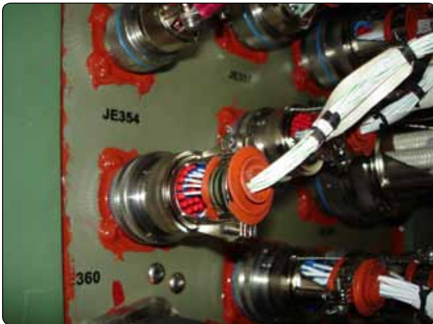
Figure 9-162. Backshells with strain relief.
