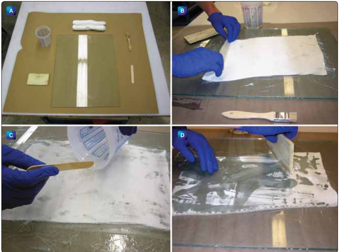
Figure 7-51. Fabric impregnation with a brush or squeegee: A) wet layup materials; B) fabric placement; C) fabric impregnation; D) squeegee used to thoroughly wet the fabric.
