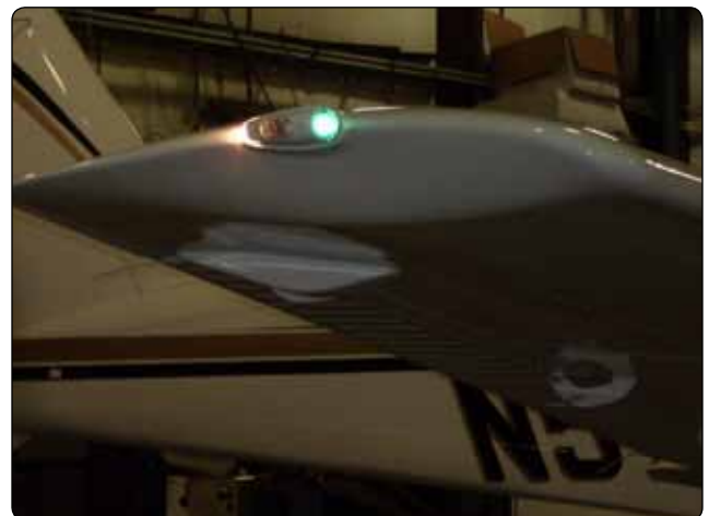
Figure 9-175. A right wing tip position light, also known as a navigation light.
