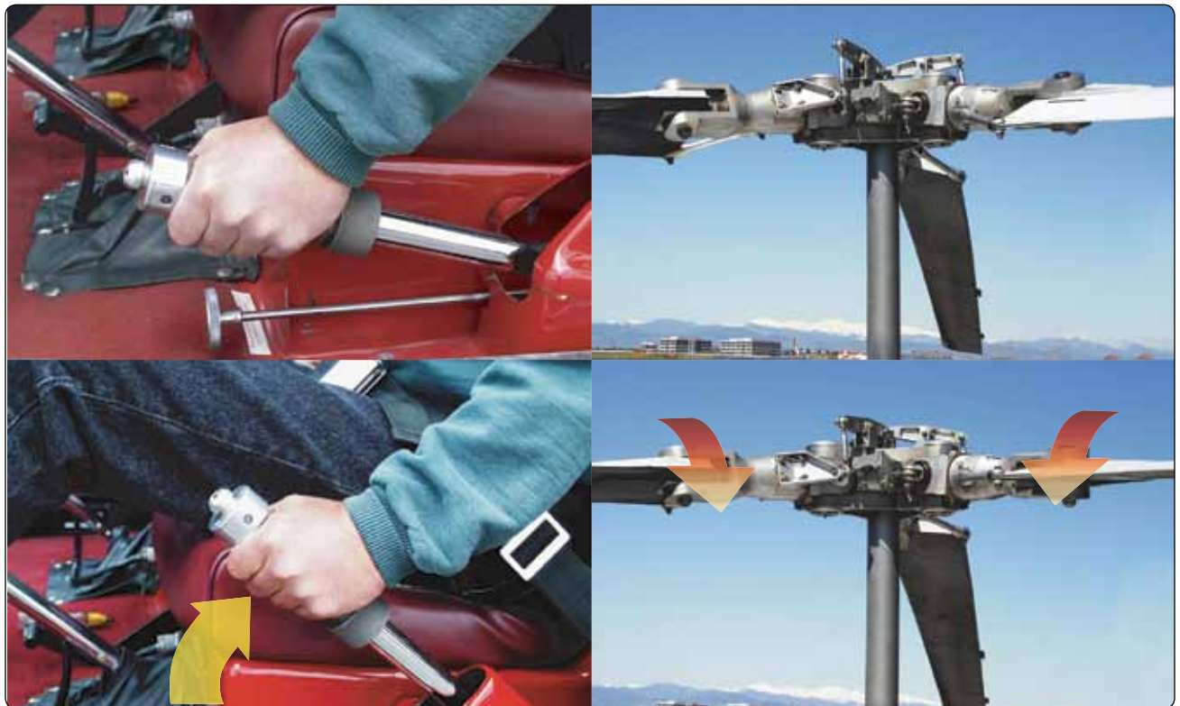
Figure 2-45. Raising the collective pitch control increases the pitch angle by the same amount on all blades.
