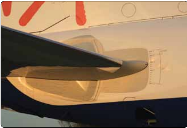
Figure 1-58. A stabilizer and index marks on a transport category aircraft.
