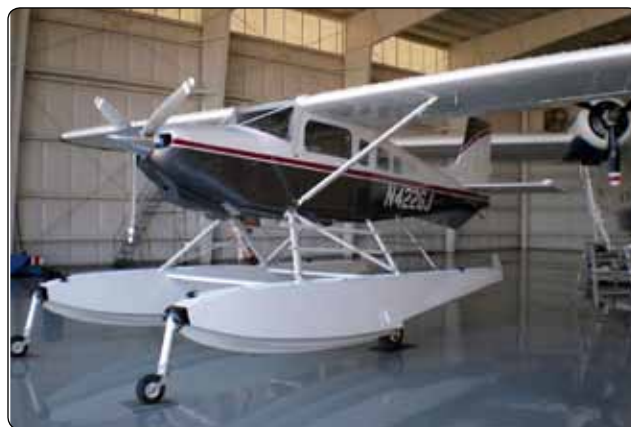
Figure 1-85. Retractable wheels make this aircraft amphibious.
