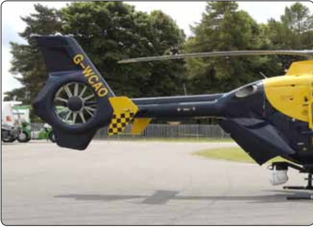
Figure 1-101. A Fenestron or “fan-in-tail” antitorque system. This design provides an improved margin of safety during ground operations.
