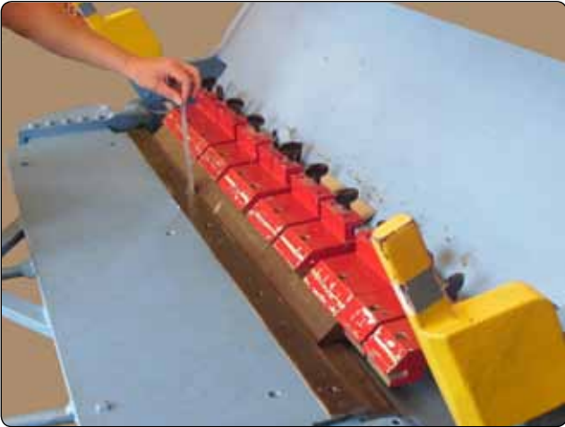
Figure 4-141. Brake nose gap adjustment with piece of material same thickness as part to be formed.
