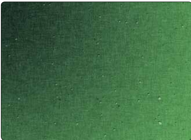
Figure 8-15. Example of pinholes.
