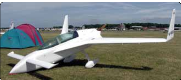
Figure 2-18. Canard wings on a Rutan VariEze.
