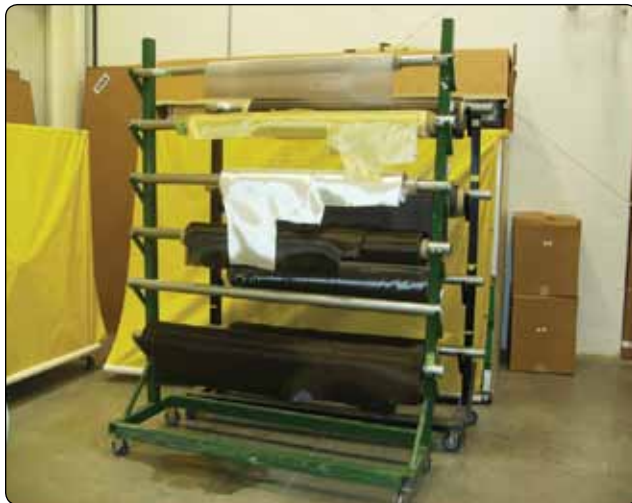
Figure 7-12. Dry fabric materials (top to bottom: aluminum lightning protection mesh, Kevlar®, fiberglass, and carbon fiber).
