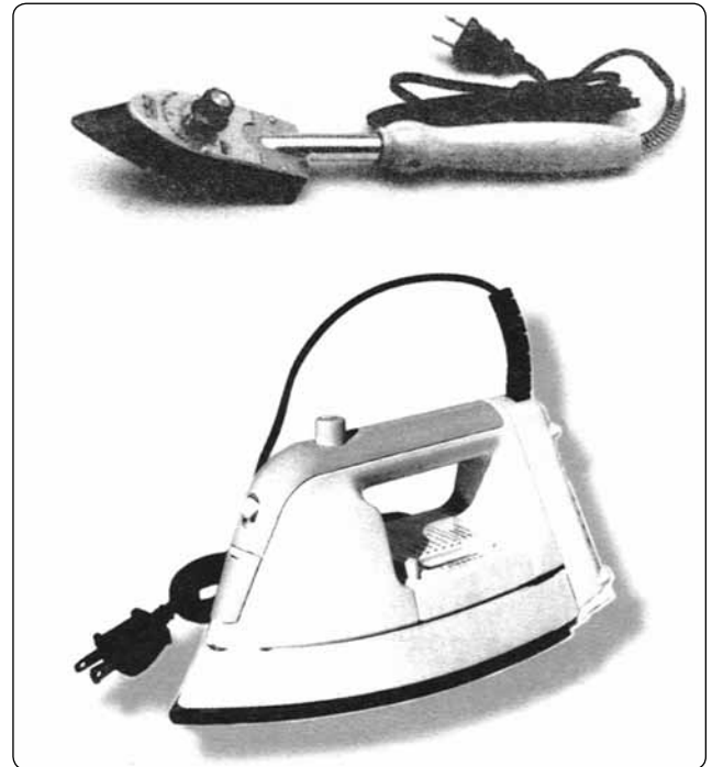
Figure 3-21. Irons used during the fabric covering process.
