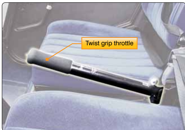
Figure 2-46. A twist grip throttle is usually mounted on the end of the collective lever. The throttles on some turbine helicopters are mounted on the overhead panel or on the floor in the cockpit.
