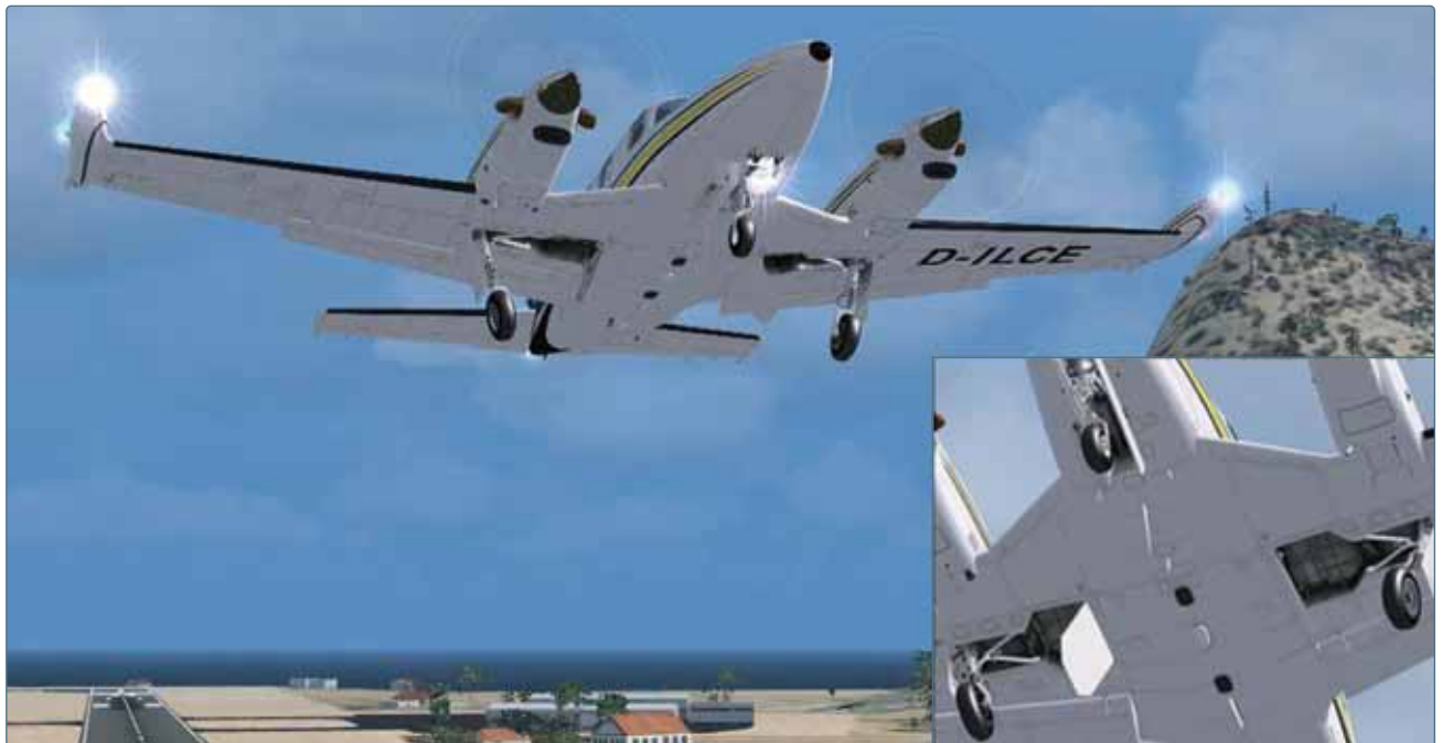
Figure 1-40. Wheel wells in a wing engine nacelle with gear coming down (inset).
