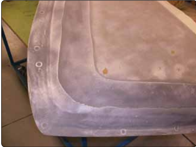
Figure 7-9. Aluminum mesh lightning protection material.
