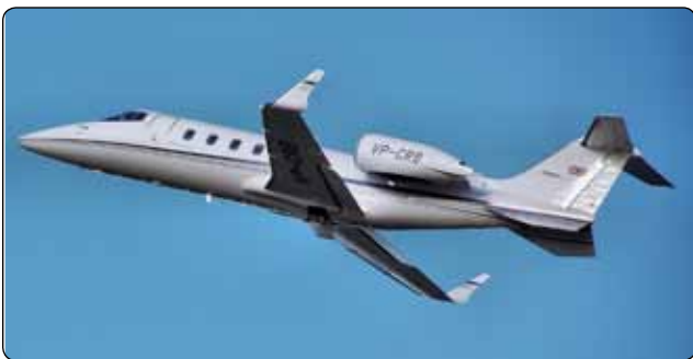
Figure 2-17. Winglets on a Bombardier Learjet 60.
