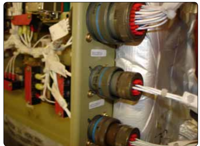
Figure 9-161. Connector arrangement to avoid wrong connection.
