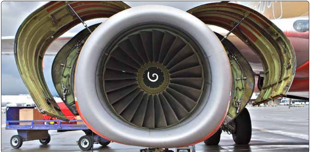
Figure 1-45. Cowling on a transport category turbine engine nacelle.
