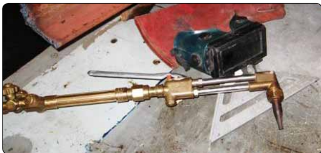
Figure 5-23. Cutting torch with additional tools.
