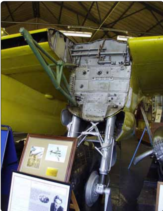
Figure 1-41. An engine nacelle firewall.
