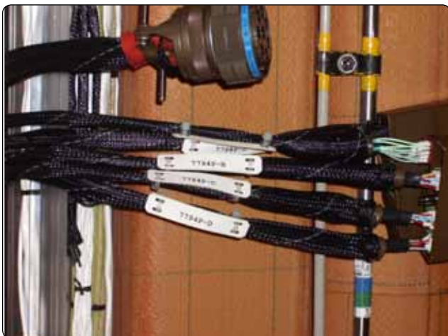
Figure 9-127. Alternate method of identifying wire bundles.
