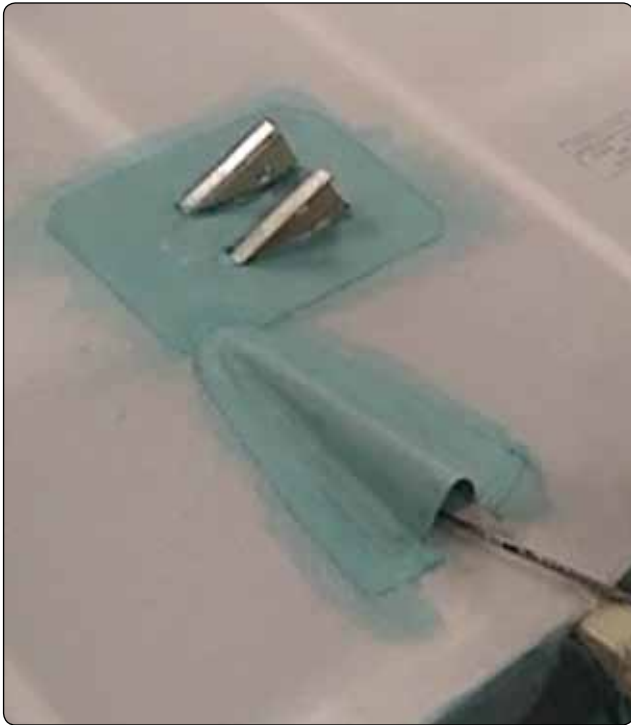
Figure 3-32. A strut fitting and cable guide with reinforcing fabric gussets cemented in place.
