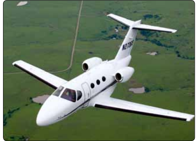
Figure 1-10. The nearly all composite Cessna Citation Mustang very light jet (VLJ).
