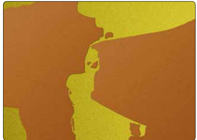
Figure 8-13. Example of poor adhesion.
