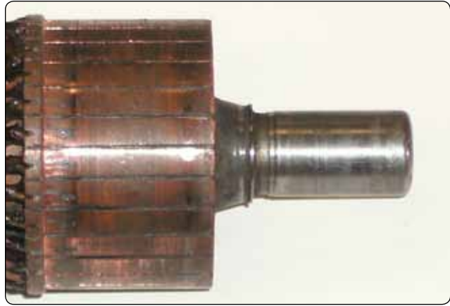
Figure 9-44. Typical DC generator commutator.
