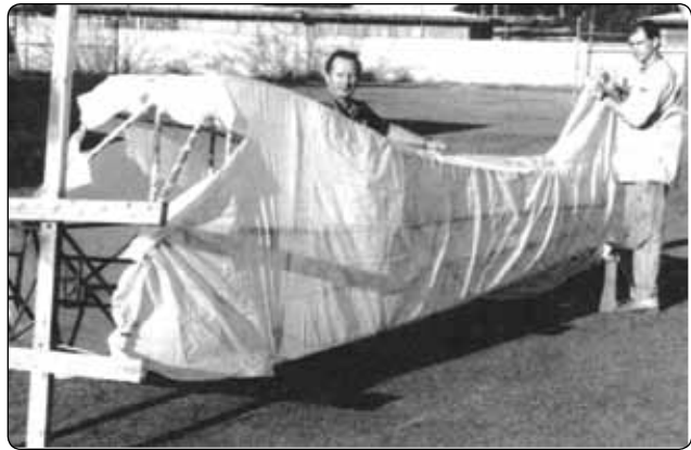
Figure 3-13. A custom-fit pre-sewn fabric envelope is slid into position over a fuselage for the envelope method of fabric covering. Other than fitting, most steps in the covering process are the same as with the blanket covering method.
