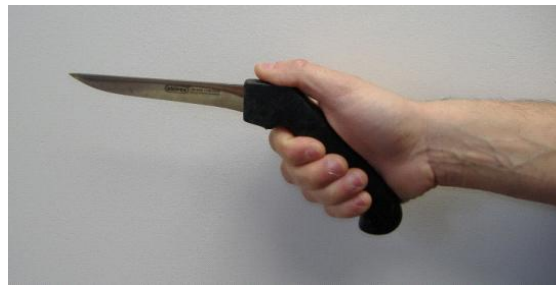
Bent angle knife for vertical cutting.
