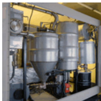
Courtesy of NREL. Small-scale gasification pilot unit.
