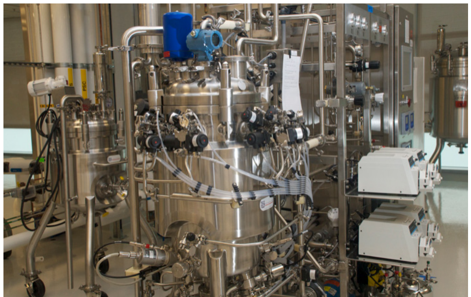
Berkeley Lab's Advanced Biofuels PDU can convert biomass into advanced biofuels in sufficient quantities for engine testing. Photo: LBNL
