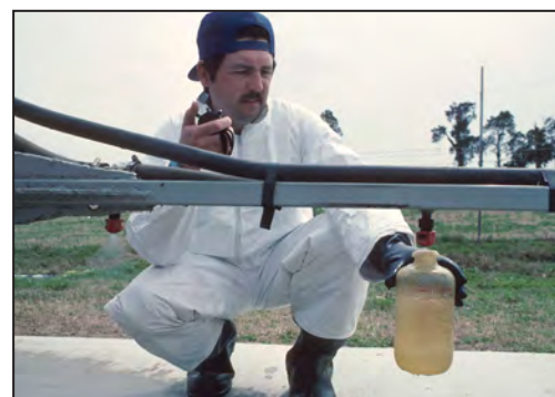
This farmer is calibrating his sprayer before applying pesticide. That action can reduce the amount of chemical used and insure that excess pesticide does not damage plants or affect surface or groundwater.
