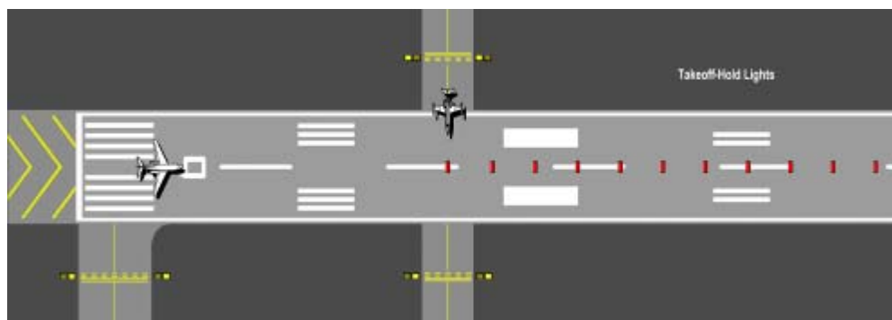
Figure 3. Diagram of Take-Off Hold Lights
