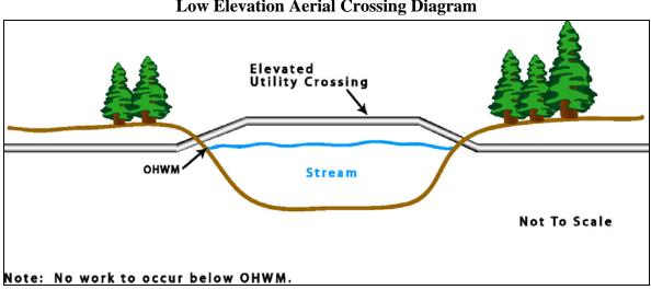
Illustration C Low Elevation Aerial Crossing Diagram
