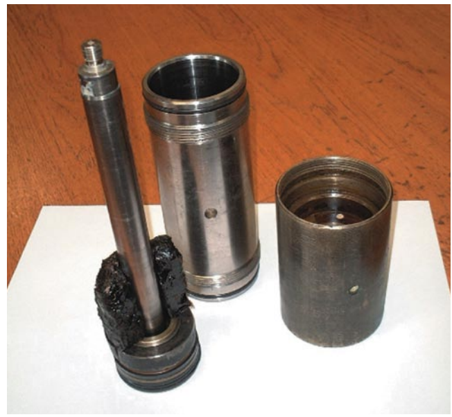
FIGURE 3-18. High-Viscosity Heavy Oil Acquired by Wireline Sampling
