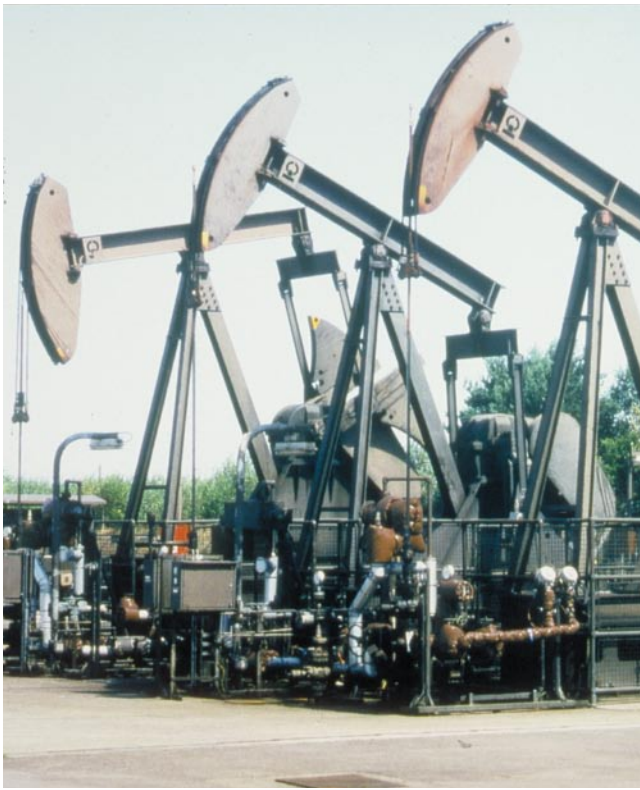
FIGURE 3-4. Pumping Units that Produce Oil from Low-Pressure Reservoirs
