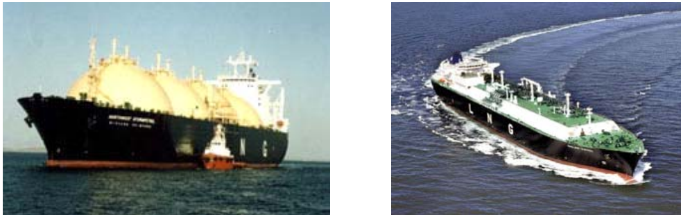
FIGURE 3-3 Sphere-type and Membrane-type LNG Tankers
