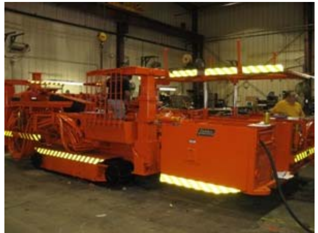
Conducting a machine audit on a roof bolter.
