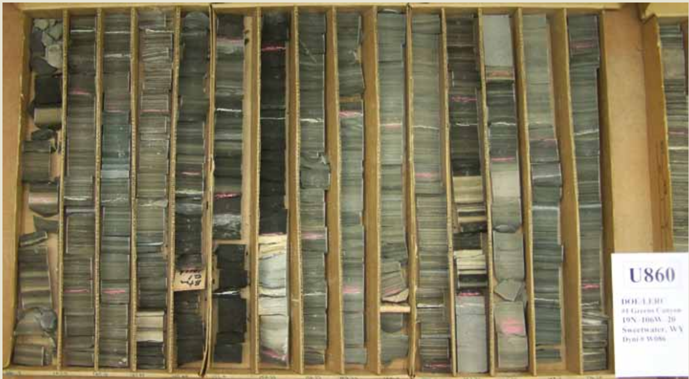
Boxes of oil shale cores from the Green River Formation in Wyoming that had been stored in the Anvil Points Mine near Rifle, Colo., and are now available for study at the Core Research Center in Denver, Colo. Photograph by Joshua Hicks, USGS.
