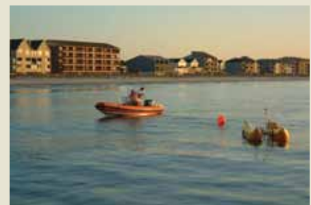
Geologists towing a subbottom profiler (yellow pontoons) in shallow water near the beach. The profiler used sound waves to provide images of the internal structure of the sea floor. From Barnhardt (2009, cover).
