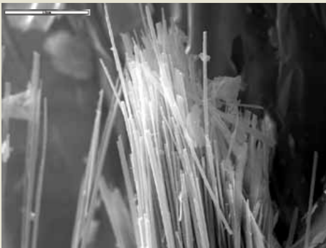
Scanning electron photomicrograph showing asbestiform (fibrous) amphiboles in vermiculite insulation produced at Libby, Mont.; the scale bar is 10 micrometers long. Photograph by G. Meeker, USGS.
