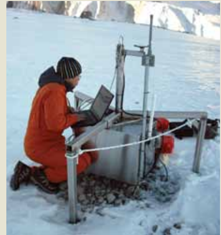
Graduate student Mingsen Xu checks on a spider (spindly frame holding an instrument) in the crater of Mount St. Helens Volcano, Wash. Photograph by Rick LaHusen, USGS, 2009.
