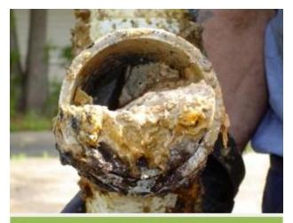
Grease can completely block sewer pipe, as shown above.
