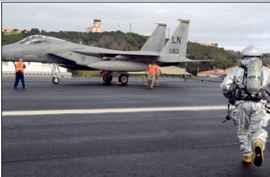
A firefighter from Lajes Field hurries to help recover an F-15C from RAF Lakenheath, England, that has engaged the base's arresting barrier during a routine test of the system Dec. 9, 2011. (Photo by Tech. Sgt. Chyrece Campbell)
