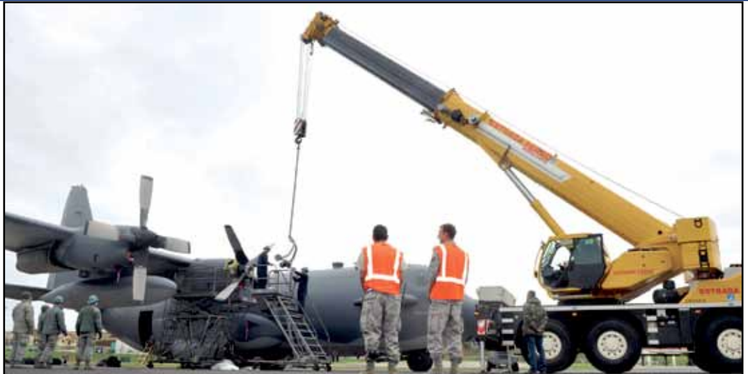
Maintainers from Cannon AFB, N.M., replace a propeller on an AC-130 Gunship after an emergency landing here over the Thanksgiving holiday. (Photos by Guido Melo)
